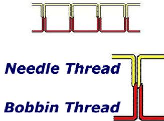
For 301 lockstitch seams, we generally recommend using the same needle thread size as the bobbin thread size in the seam. Why? Because “a chain is only as strong as its weakest link.” If a smaller, weaker thread is used in the bobbin, then the seam will only be as strong as the bobbin thread. This is particularly true with lockstitch seams because of the way the needle and bobbin threads are interlocked together.
